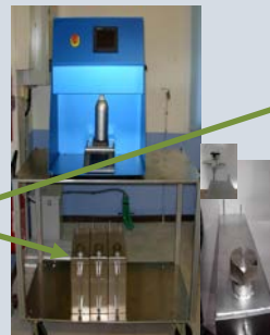
Blender without burettes & Pumps / Blender with burettes (Gravity)
